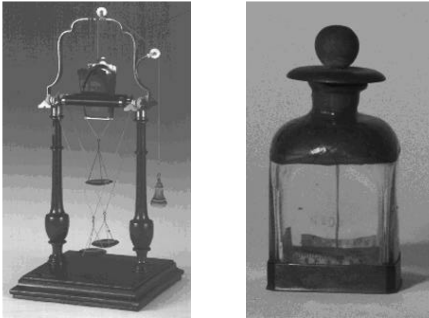
Figure 11 Re's wedge demonstration and straw electrometer probably made by him (courtesy Liceo "Ugo Foscolo" and MSUPV).
