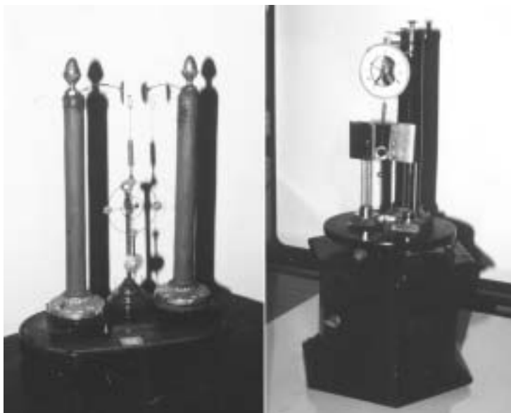
Figure 6 Two Zamboni realizations: on the left picture the pendulum (perpetual electromotor) kept in Verona College “S. Maffei”, and on the right picture the clock supplied by dry piles, kept in Mantua College “Virgilio”.
