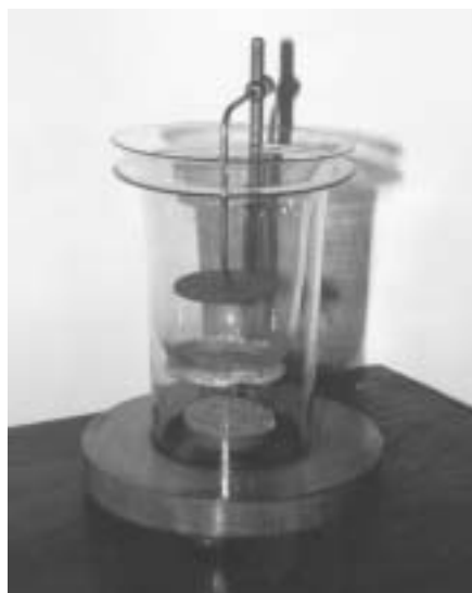
Figure 5 A disassembled model of the cell unit of Zamboni's dry pile for didactical use.
