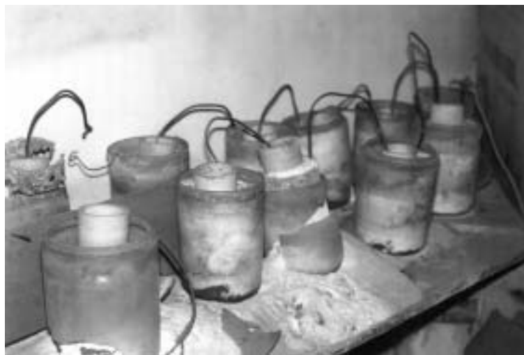
Figure 4 The battery of Candido's piles that powered the electrical tower-clocks of Lecce from 1868 to 1936, as found in 1990 (picture by L. Ruggiero).
